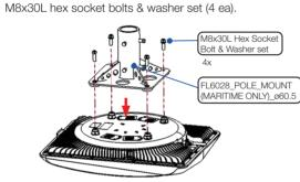
4. Once ODU and the pole mount is secured, assemble it onto the 60mm pole and push in to the end of the adapter hole.
