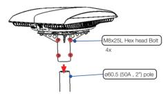
Secure the pole and the pole adapter using M8x25 hex socket bolts (4ea). Tighten the four bolts to securely push the pole surface back with inner pole mount surface.
