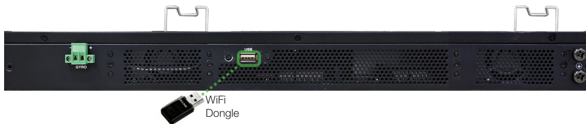
Figure 49: Back Panel Wi-Fi Dongle Connection
