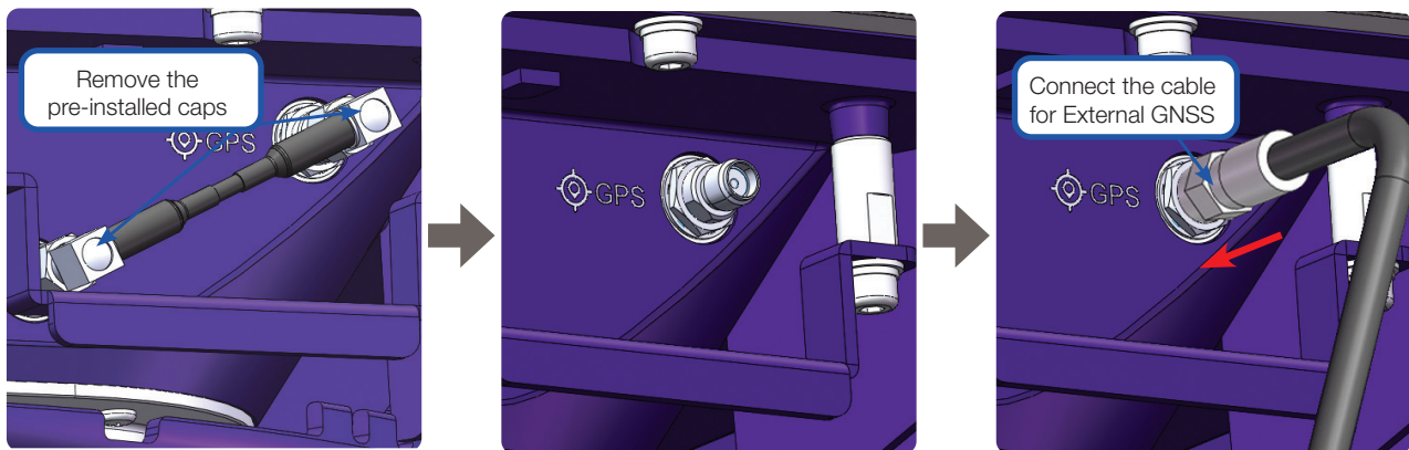
Figure 32: Connecting the SMA connector of the external GNSS cable to the GNSS connector
