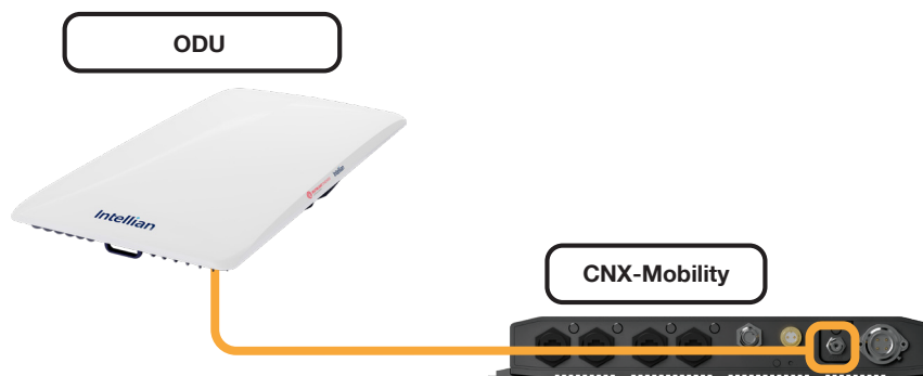
Figure 62: Connecting Power to CNX-Mobility
