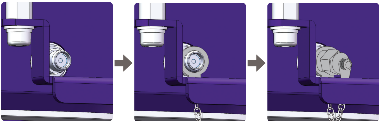
Figure 33: Close the left-hand connector (without GPS sticker) using the SMA cap provided
